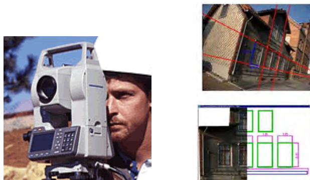
Examples of architectural documentation: surveying with a total station (left), creating drawings from rectified photographs (right)
