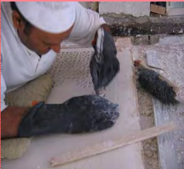
Nagui carving a new gypsum window.
